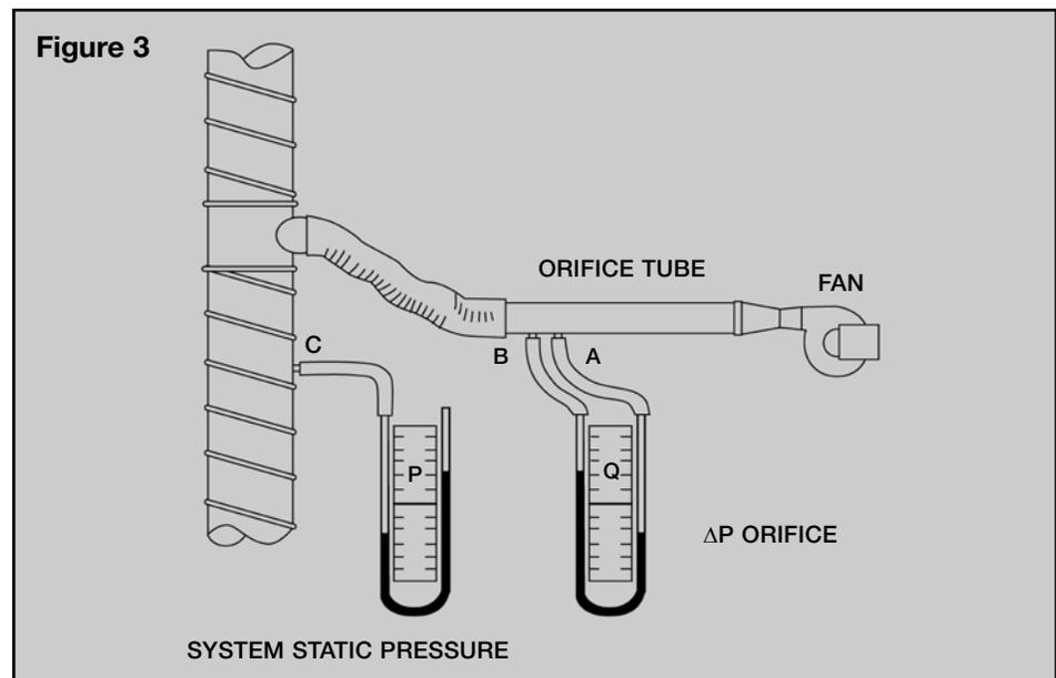
**Step 9** — Using additional plastic tubing, connect either side of the other manometer to tap A, and the other side of this manometer to tap B on the orifice tube. This manometer, identified as “Q” in **Figure 3**, will measure the differential pressure across the orifice plate. Check the manometer’s water level again and adjust it to zero, if necessary.
