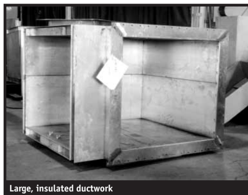
Large, insulated ductwork
