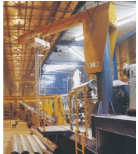
Each mobile unit is equipped with a 2-ton overhead crane for easy and convenient material handling.
