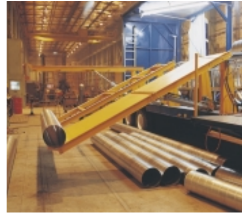
Each Mobile Duct Machine uses a pneumatic or hydraulic handling table, which allows the operator to deliver the duct directly into the hands of the contractor.
