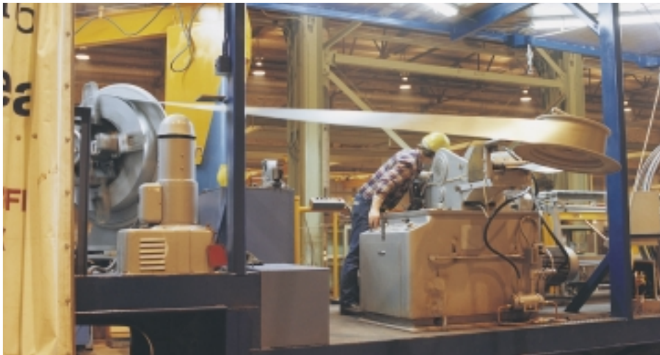
Each self-contained Mobile Duct Machine is equipped with an air compressor, welding machine, steel decoiler, heating, and lighting. A separate truck-mounted electrical generator is also available.
