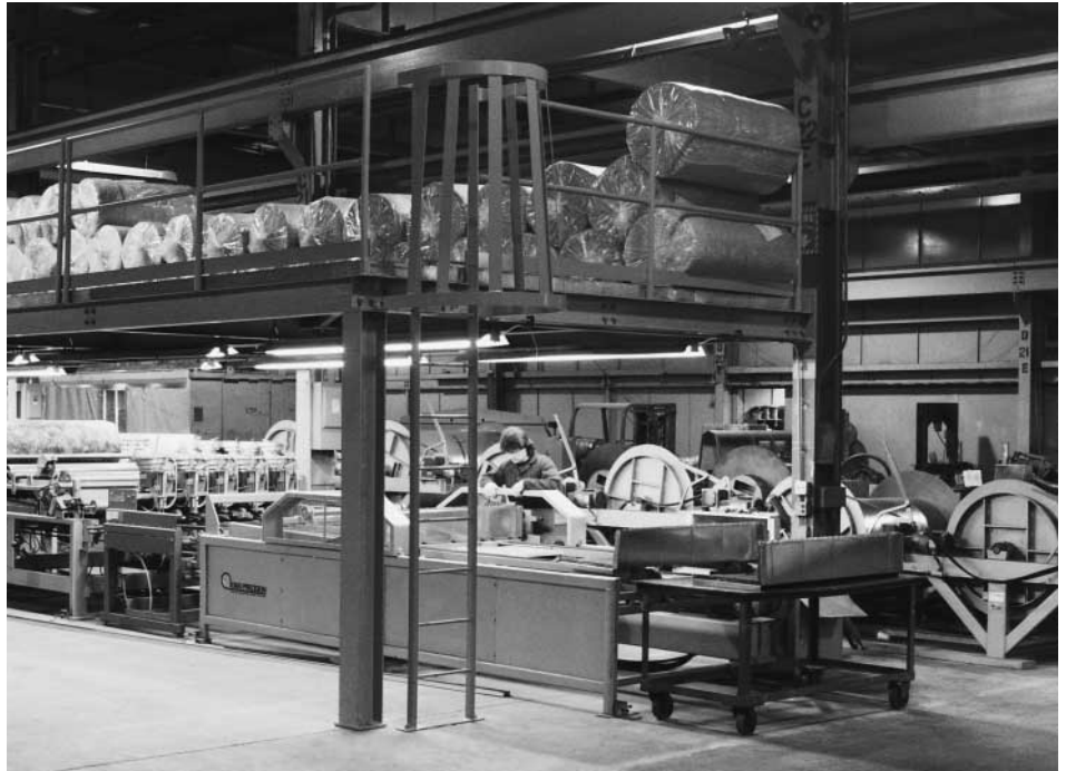
Automated coil lines enable us to produce rectangular duct economically.
