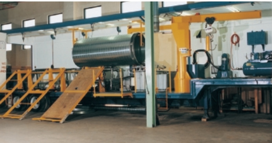
McGill's Mobile Duct Machine is a self-contained, 42-foot trailer with an air compressor, welding machine, steel decoiler and a two-ton, overhead crane. A pneumatic handling table delivers the duct directly to the contractor.
