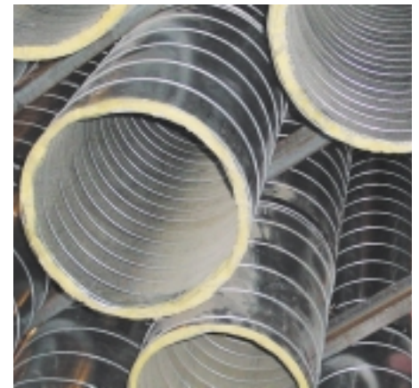
Double-wall duct construction protects the fiberglass insulation during cleaning and inhibits entrainment.
