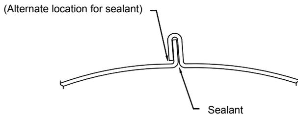
Sealed with United Duct Sealer™ (Water Based)
