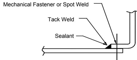
Sealed with United Duct Sealer™ (Water Based)
