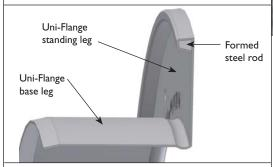
Uni-Flange connectors incorporate a formed, solid cold-rolled steel rod in the standing leg for additional rigidity, which is especially good for flat oval and large diameter duct. This also helps protect product integrity under rough shipping and handling conditions.
