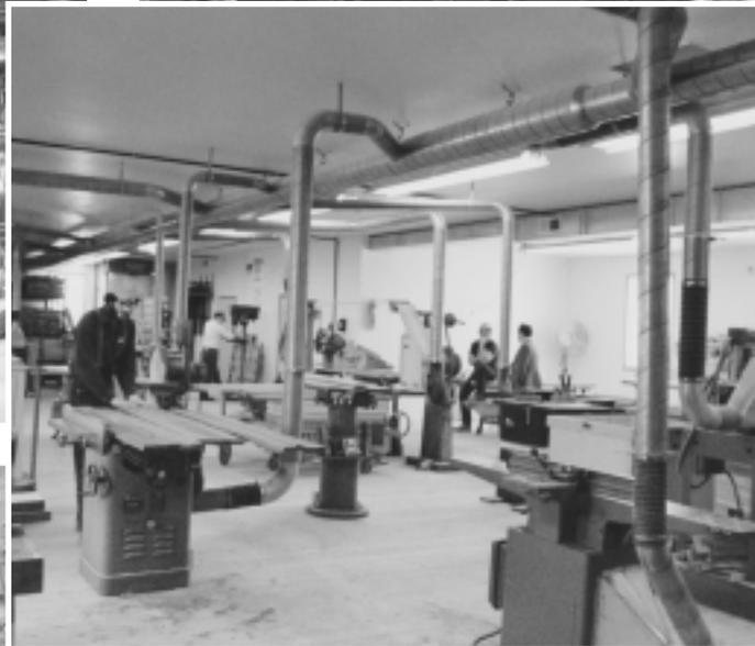
Dust control and particulate conveyance (woodworking)
