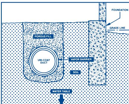
but is not beneath or encased in concrete. The installation procedure is the same as for under-slab, below grade. Make sure that at least 12 inches of compacted cover exists. Any equipment that can cause point loads above the ductwork (even light loads) must not be operated near the area.
