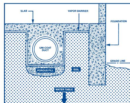
The duct, either encased in concrete or buried directly below a concrete slab, is installed above the original line of undisturbed soil and above the water table. Encasing the duct in concrete with a porous fill beneath it is the best way to install UNI-COAT duct. An appropriate vapor barrier (e.g., 4 mil polyethylene) must be placed between the duct and the concrete.
