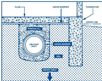
Heavy equipment such as bulldozers and loaded dump trucks must not be operated near the site until there is at least 5 feet of compacted cover. Bridging is required if maximum loading is exceeded. Refer to McGill AirFlow's Engineering Report No. 155 when determining maximum depth of burial.
